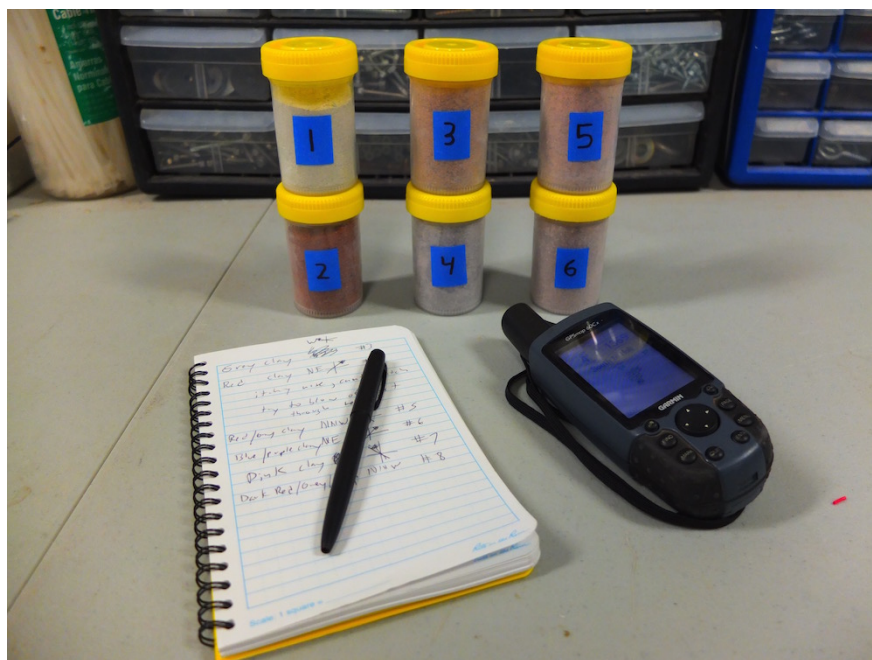
Figure 5.14: Colored pigment soil samples collected at the MDRS by the author. Each sample was documented with photos and a GPS coordinate.
