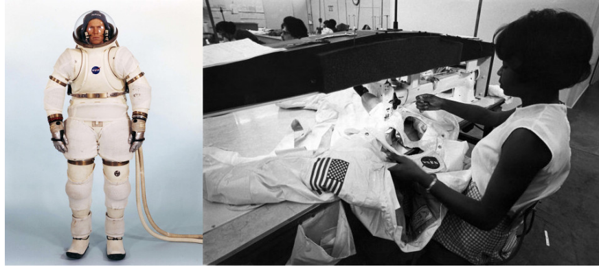
Figure 3.3: (left) Litton RX2A Apollo hardsuit prototype favored by NASA 1965 (right) Apollo A7L Thermal Micrometeoroid Garment layer on the ILC assembly line
